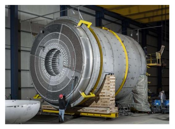
Pic. 14: MBRF-Heat-Exchanger for Zn-Roasting Plant
